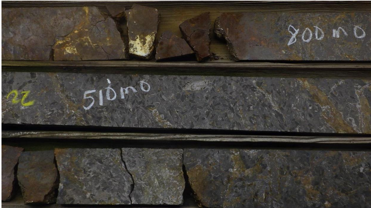
Photo A: graphitic schist with 20% Cg and Mo, Ni, Zn and Ag mineralization from 22-23m.
