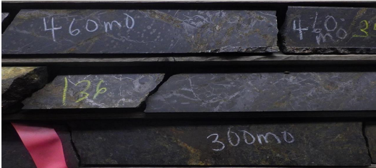
Photo C: 34.9% graphitic carbon in the sample from 36 to 37m - brecciated graphitic schist.
